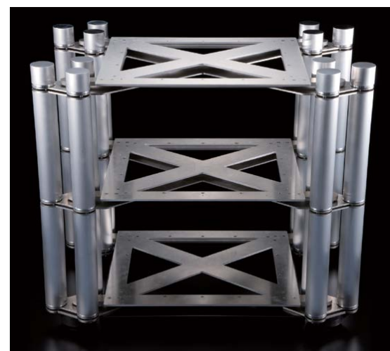
Aluminum board on top of the Full-Con mech of the 4 corners. This board moves in horizontal directions. Another aluminum board underneath of that is the frame to stabilize the pillars of the 4 corners and is combined with the upper board by a spike mechanism.
