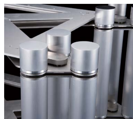
Aluminum board on top of the Full-Con mech of the 4 corners. This board moves in horizontal directions. Another aluminum board underneath of that is the frame to stabilize the pillars of the 4 corners and is combined with the upper board by a spike mechanism.
